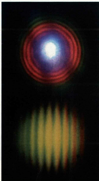
DIFFRACTION, as occurs when a wave emerges from a small aperture, can influence supercontinuum generation. At the top, diffraction of a near-infrared laser beam through a 300-micron hole and onto a nearby glass slide produces a spot intense enough for supercontinuum generation [white]. At the bottom, light diffracted by a straight edge generates supercontinuum light from two spots. The two beams interfere with each other, producing lines.
