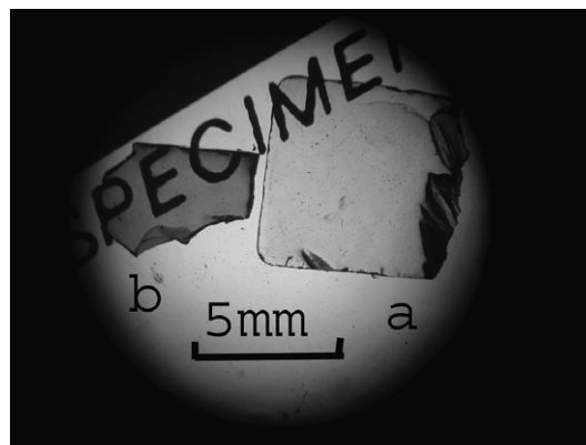
Fig. 2. Optical microscopy picture of parent glass (a) and glass-ceramic (b) samples (glass composition #7, as-quenched and after heat-treatment at 525 °C for 1 h).
