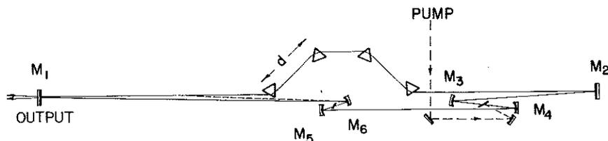
Fig. 1. Schematic diagram of the linear ring cavity CPM dye laser employing an almost-normal incidence angle. The dashed line represents the possibility of adjusting the cavity length, which is easily achieved by moving mirror  $M_1$  and making a minor adjustment to mirror  $M_6$ .
