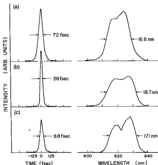
Fig. 2. Autocorrelation functions and their corresponding spectra for three different Kiton Red concentrations in a Rhodamine 590-ethylene glycol solution (Rhodamine 590 concentration of  $1.6 \times 10^{-3} M$ ). (a) No Kiton Red, (b)  $3.9 \times 10^{-5} M$  Kiton Red, (c)  $7.1 \times 10^{-5} M$  Kiton Red.
