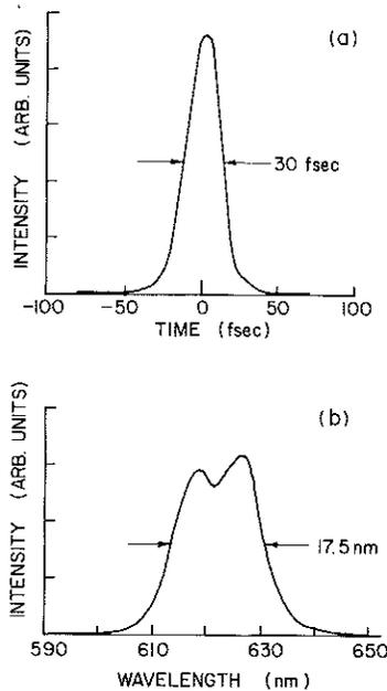
Fig. 4. (a) Autocorrelation trace of pulses having 30-fsec duration and (b) corresponding spectrum obtained for optimum Kiton Red-Rhodamine 590 solution when DODCI concentration was also optimized (DODCI concentration of  $1.3 \times 10^{-4} M$ ).
