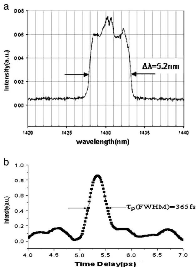
**Fig. 4.** (a) Measured autocorrelation trace of the mode-locked Cunyite laser Spectrum of the mode-locked pulses; (b) Central wavelength  $\lambda_c = 1430$  nm, bandwidth  $\Delta\lambda = 5.2$  nm, and pulse width  $\Delta\tau = 365$  fs. Circles represent experimental data and the solid line is the best fit corresponding to  $\text{sech}^2$  pulse shape. FWHMs are shown by arrows.
