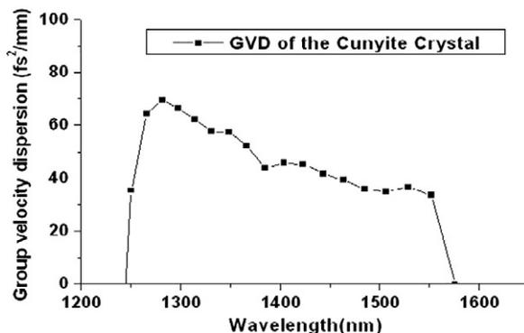
Fig. 3. Group delay dispersion (GDD) of a 3-mm Brewster cut  $\text{Cr}:\text{Cunyite}$  sample. Points represent measured values.
