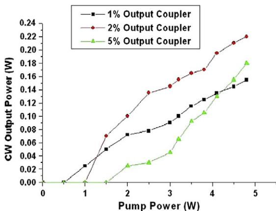
Fig. 2. CW efficiency curves for the Nd:YAG pumped  $\text{Cr}:\text{Ca}_2\text{GeO}_4$  (Cunyite) laser taken with the 1%, 2.5%, 5% OCs.
