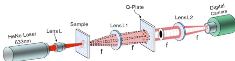
FIG. 1. Diagram of the 4f q-plate dark field OAM microscopy setup.
