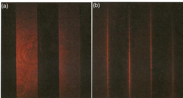
FIG. 3. Metal bars without voltage (a) and with voltage (b) on the q-plate in the 4f system.
