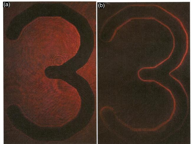
FIG. 4. Opaque number 3 without voltage (a) and with voltage (b) on the q-plate in the 4f system.
