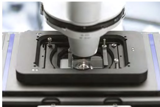
Z piezo stage and a leveling insert guarantee the precision needed for superresolution applications using ZEISS Airyscan.
